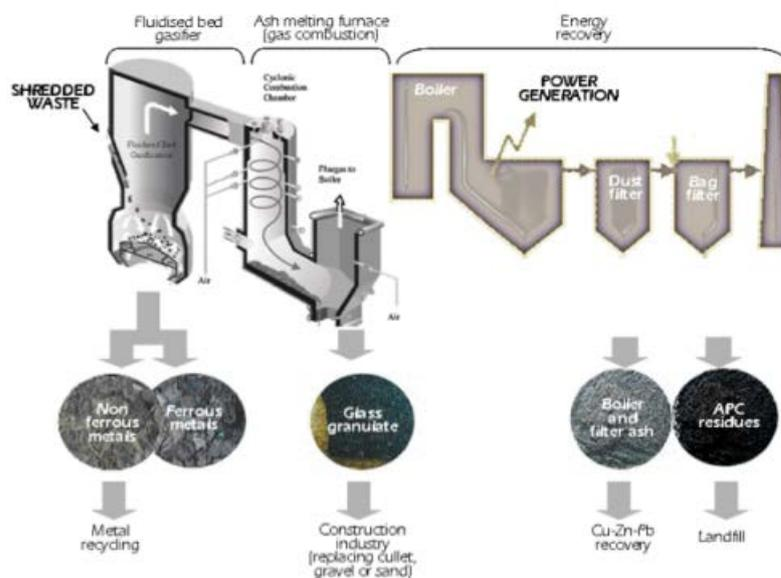
Figure 8: Slagging Gasification / Fluidised Bed Gasification Process
