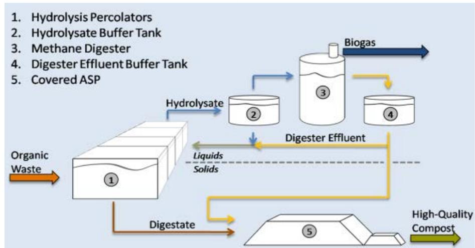
Figure 12: MBT B Process Flow Diagram
