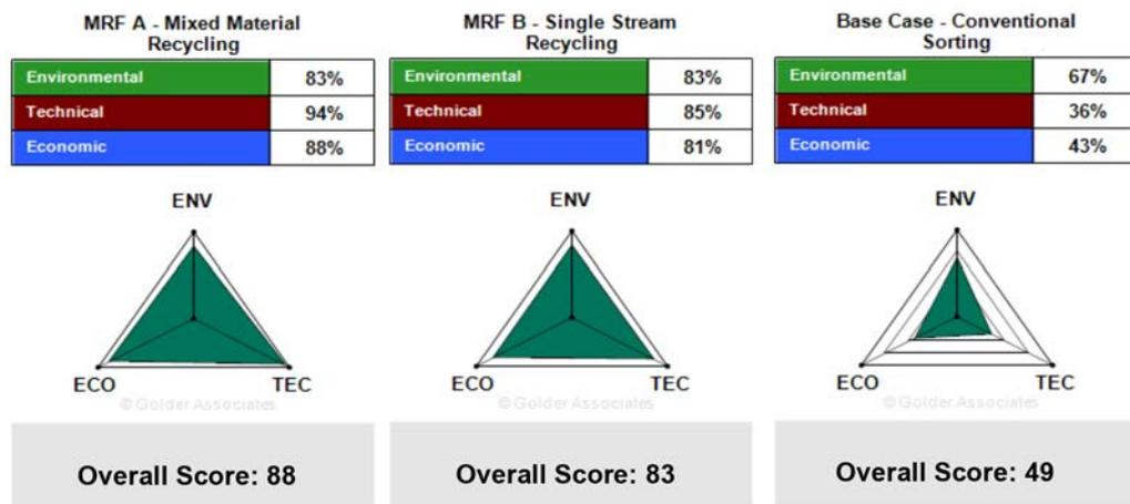
Both MRF A and MRF B show significantly better performance than the base case of conventional manual sorting facility. MRF B has similar results as MRF A with moderate to high beneficial environmental, technical and economic outcomes.
