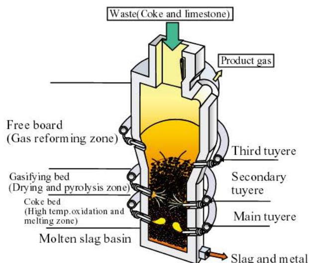
**Figure 6: Slagging Gasification - Shaft Type**
