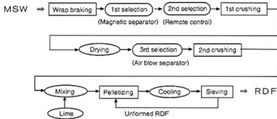
Figure 11: Typical MBT A Process Flow Diagram
