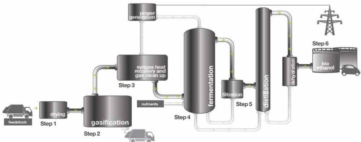
Figure 13: MBT C Process Flow Diagram
