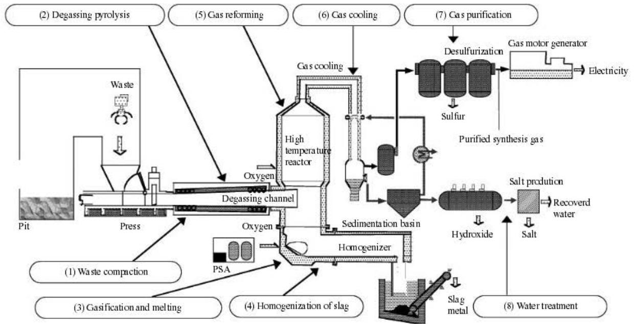
**Figure 5: Pyrolysis + Gasification Process**
