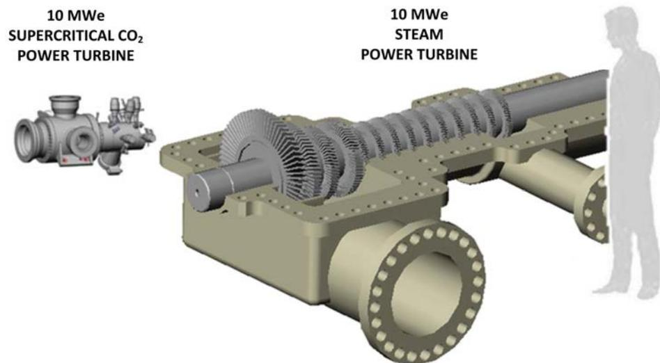
Suitable fluids for these applications have relatively low critical temperatures and pressures, so they can be compressed and heated directly to their supercritical state before expansion, which enables a better thermal match with the heat source.
