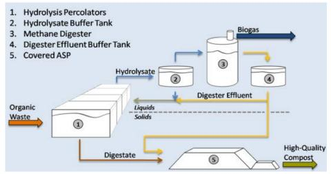
Figure 12: MBT B Process Flow Diagram
