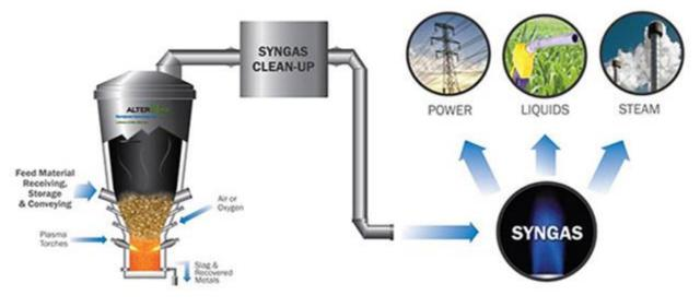
Figure 7: Gasification + Plasma Process
