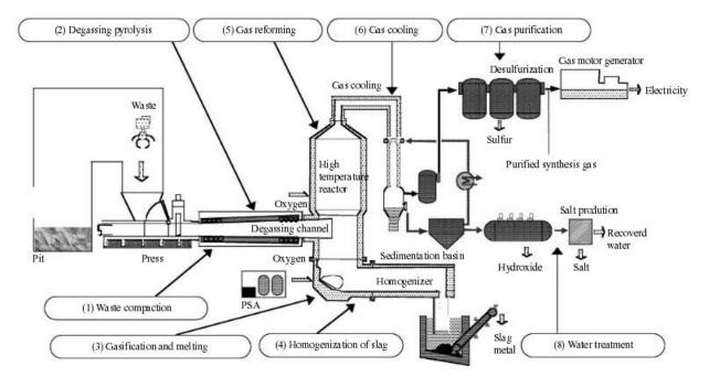
Figure 5: Pyrolysis + Gasification Process
