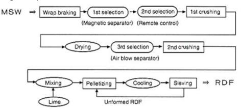
Figure 11: Typical MBT A Process Flow Diagram
