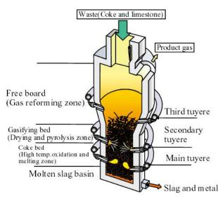
Figure 6: Slagging Gasification - Shaft Type
