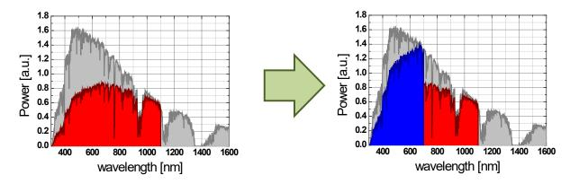
*Figure 5.5:* Generic principle of better harvesting the solar spectrum through double junction solar cells (tandems)
