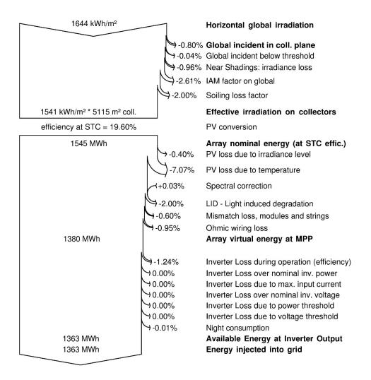
Figure 5.8: PR loss analysis of a typical PV system deployed in Singapore (using PV Syst software).
