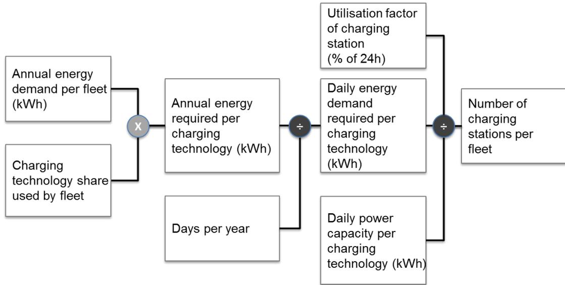
**Figure 21 Method to Calculate the Annual Number of Charging Stations Required per Fleet**
