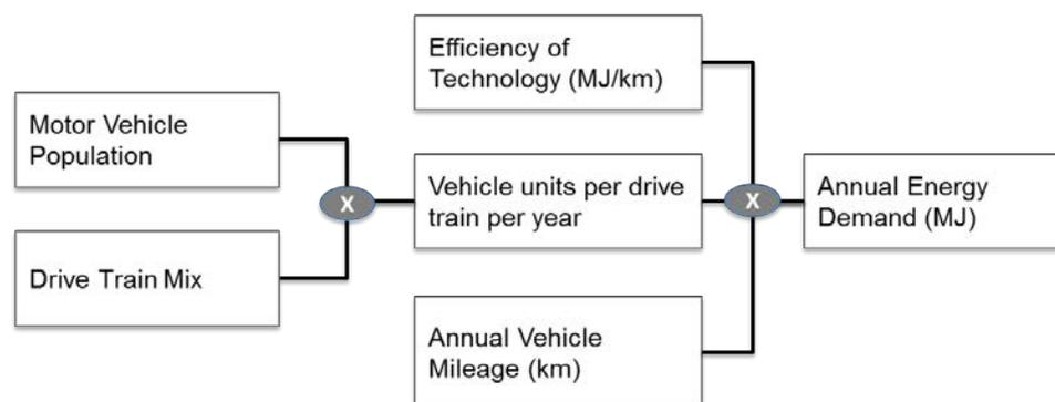
**Figure 18 Method to Calculate the Annual Energy Demand of a Fleet**
