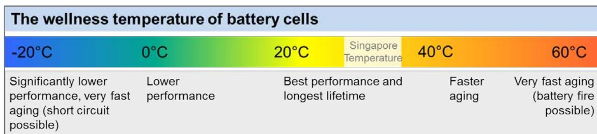
**Figure 8: Wellness Temperature Range for Battery Cells**
