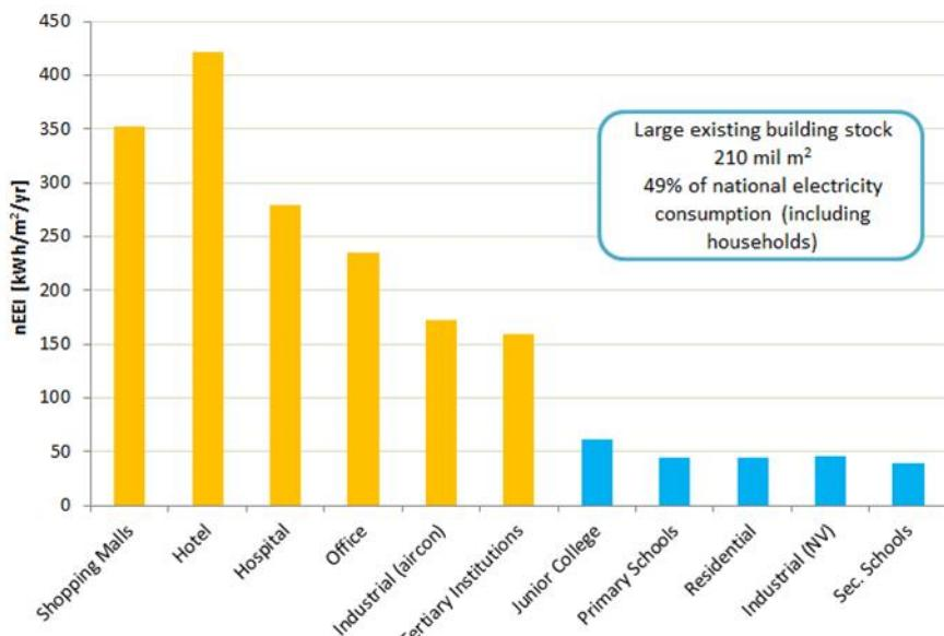
Figure 1.2: Energy consumption in existing building types (BCA, 2012a)
