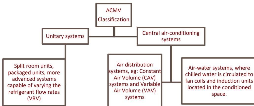
Figure 2.4: Unitary and central air-conditioning systems in Singapore (Aircon Primer, 2011)
