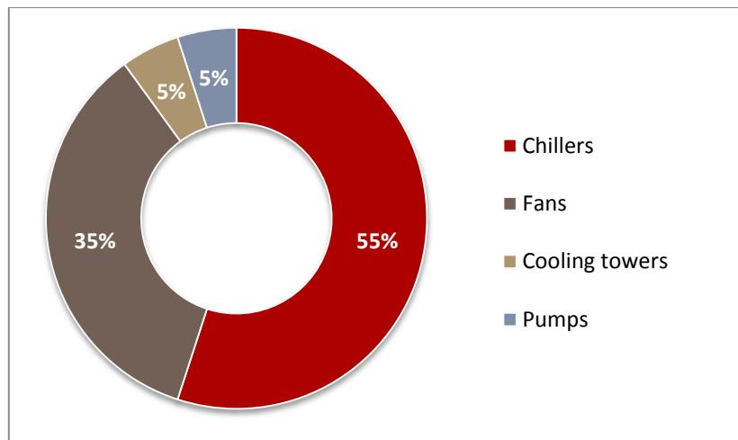
**Figure 2.3: Energy consumption breakdown for ACMV Systems (Aircon Primer, 2011)**
