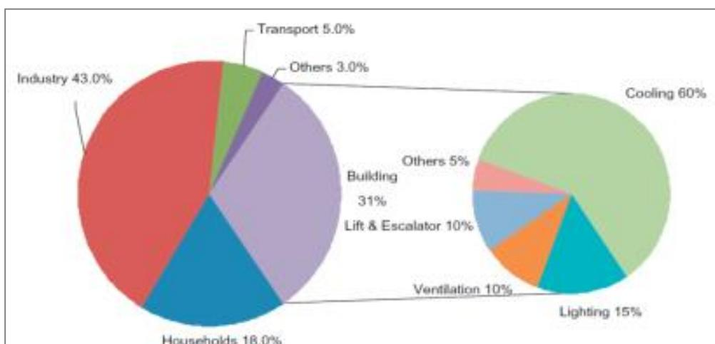
Figure 1.3: Typical electricity consumption by end-use in Singapore and in the building sector (Chua et al., 2013)
